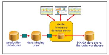
Figure 6 HANA as a replacement for the enterprise data warehouse database and the derived databases, such as data marts and personal data stores
