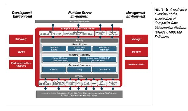
Figure 15 contains a diagram that shows the architecture of the Composite Data Virtualization Platform and includes most of the data stores that can be accessed and most of the API's being supported.
