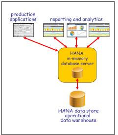
Figure 8 Operational Bl in which one database acts as production database and as data warehouse
