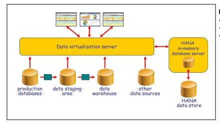
Figure 13 In this architecture HANA is used by the data virtualization server to speed up access to the cached virtual tables
