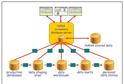
Figure 5 HANA can be used as a performance booster in an existing BI system; the symbol - represents an ETL or replication process
